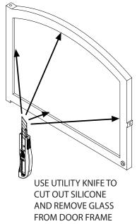
2. Un-latch the door and swing it wide open to access the glass.
